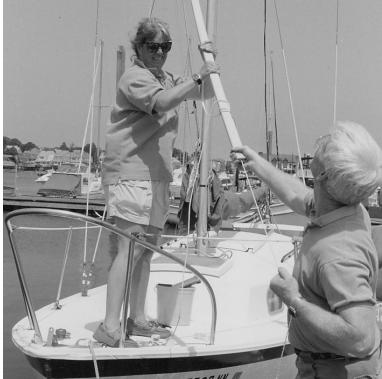
pushing extrusion up forestay
