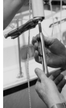
screwing turnbuckle on stud
