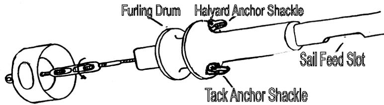
11. Slide the furling drum over the luff with the sail feed slot on the same side as the tack anchor shackle (see drawing above). You may knock the thrust washer (part "M" on page 2) out of place doing this. You can push the washer up into the cavity of the furling drum again. The washer is designed to ride between the furling drum and the plastic bearing.
