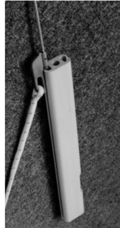
Inserting FF6 traveler into top of luff
