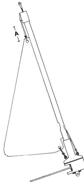
Note: When the sail is UP, the FF4 ferrule (little metal tube swaged on halyard) or FF6 traveler is DOWN near the spool.
