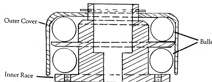
The ball bearing should be rinsed occasionally with fresh water. If the bearing is hard to turn, disassemble for a more thorough cleaning. To do so:
