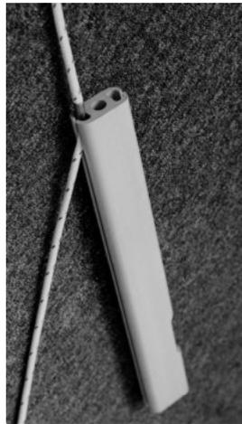
Inserting FF4 ferrule into top of luff
