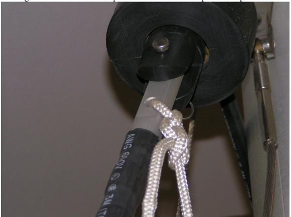
3. With a short piece of ¼" dia. double braid line, attach the tack of the spinnaker to the holes in the spinnaker swivel. (see picture). The length of line used will help determine the sail shape of the spinnaker.
